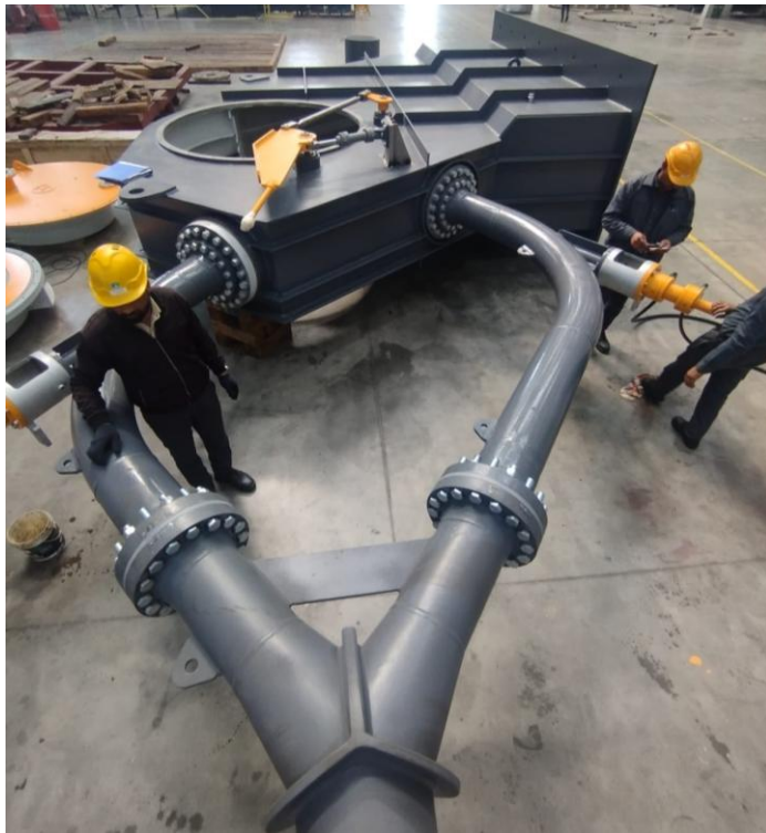
Photo 9-51 Ypiece, branch pipes and turbine housings
