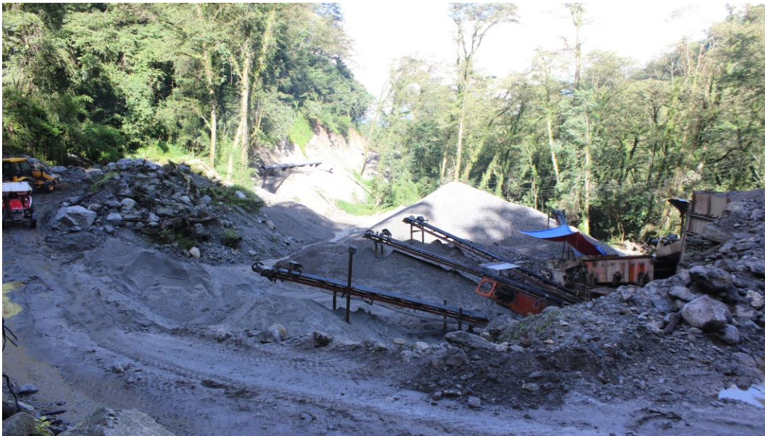
Photo 9-10 Crusher setup and aggregate production
